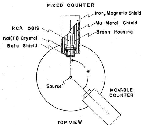
FIG. 1. Top view of scintillation spectrometer table. The details of the magnetic shielding of the photomultiplier tube and the  $\beta$  shields of the crystals are shown.
