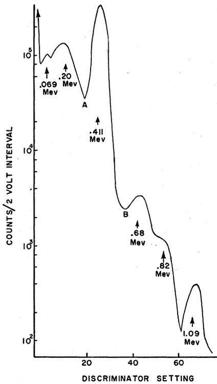
FIG. 2. Differential pulse-height distribution of pulses produced in NaI crystal by  $Au^{198}$   $\gamma$  rays.
