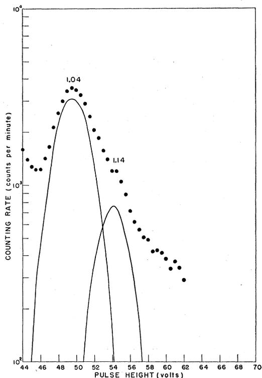
FIG. 2. Pulse-height spectrum of Rh<sup>106</sup> between 0.90 and 1.30 Mev on NaI(Tl) scintillation spectrometer. Distance from crystal 27.5 cm; activity 1.13 × 10<sup>10</sup> disintegrations/min; gain 4.
