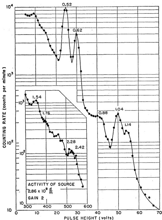
FIG. 1. Pulse-height spectrum of  $\text{Rh}^{106}$  between 50 keV and 2.50 MeV on NaI(Tl) scintillation spectrometer. Distance from crystal 2.45 cm; activity  $1.11 \times 10^7$  disintegrations/min; gain 4.
