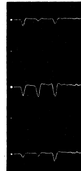
FIG. 4. Photographic records of three shower events showing the pulses from the three scintillation counters.
