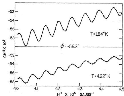
FIG. 1. Arsenic:  $CH^{-2}$ , the couple per unit mass in dyne-cm per gram acting on the crystal divided by the square of the magnetic field, versus the reciprocal of the magnetic field.
