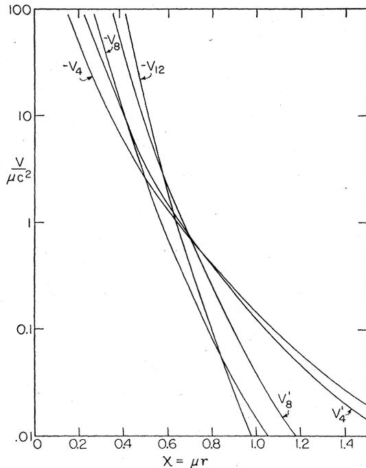
FIG. 1. Plot of the leading terms of the fourth-, eighth-, and twelfth-order potentials for  $g^2/4\pi=10$ . The unprimed potentials are generated by matrix elements with the maximum number of pairs, the primed potentials by matrix elements with one pair fewer.
