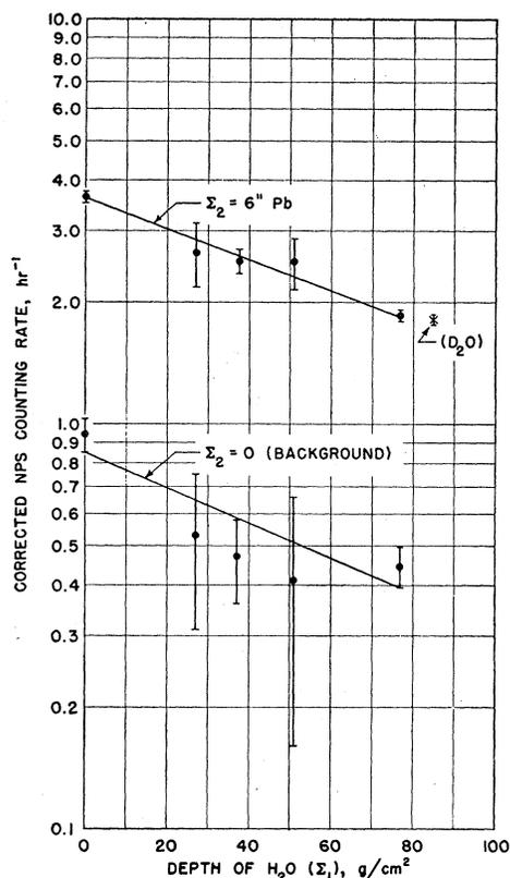
FIG. 4. Absorption of neutral  $N$  rays by light water.
