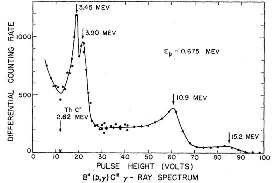
FIG. 3. Pulse-height distribution at the 0.675-Mev resonance.
