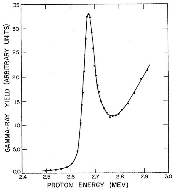
FIG. 8. Excitation curve for the reaction  $B^{11}(p, p'\gamma)B^{11}$ .  $E_\gamma = 2.13$  Mev.
