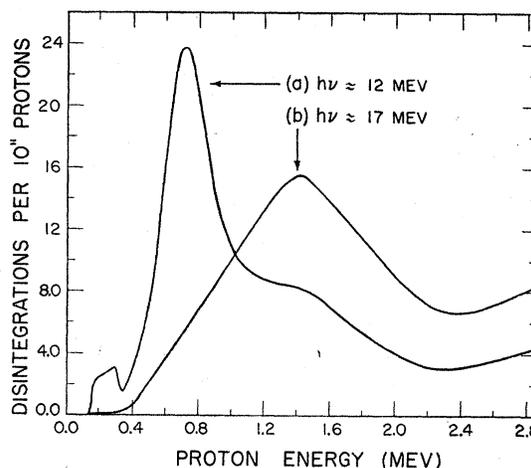
FIG. 6. True yield curve for the capture radiation, obtained from Fig. 1 by applying the corrections described in the text. The target thickness at the three resonances is given in Table II. Except at the lowest-bombarding energies, the distortion of the shape of the curve by the target thickness is small.
