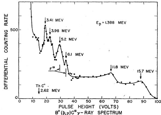
FIG. 4. Pulse-height distribution at the 1.388-Mev resonance. The peaks at 5.2 Mev and 6.1 Mev are probably from the  $F^{19}(p, \alpha\gamma)O^{16}$  reaction.
