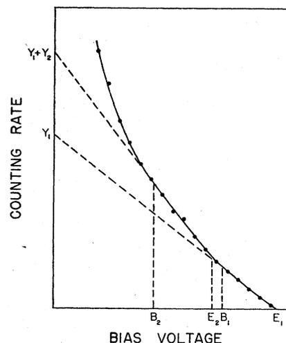
FIG. 5. Typical integral bias curve for B<sup>11</sup>( $p, \gamma$ )C<sup>12</sup>.  $E_1$  and  $E_2$  are the end points of the two high-energy gamma rays.  $Y_1$  and  $Y_2$ , which are the total number of pulses from each gamma ray, are obtained by extrapolating the corresponding straight portion of the curve linearly to zero bias.  $B_1$  and  $B_2$  are the biases used in obtaining the curves in Fig. 1.
