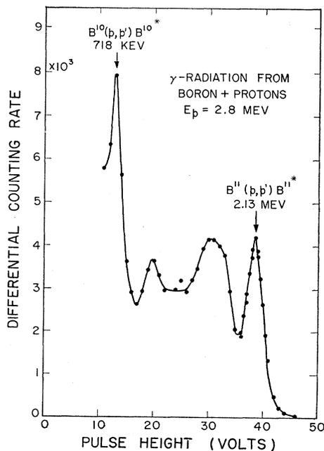
FIG. 7. Pulse-height distribution obtained at a bombarding energy of 2.8 Mev for the gamma radiation resulting from inelastic scattering.
