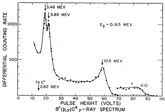
FIG. 2. Typical pulse-height distribution at the 0.163-Mev resonance.
