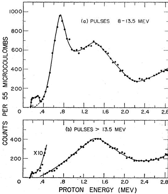
FIG. 1. Variation of yield with bombarding energy. (a) Pulses from the scintillation counter corresponding to secondary electron energies from 8 to 13.5 Mev. (b) Pulses corresponding to energies greater than 13.5 Mev.
