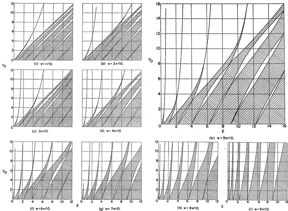
FIG. 2. Band structure as a function of energy and well depth. In (e), note the recrossing of the boundary curves which share the exceptional point  $E=6.25$  on the  $E$  axis.
