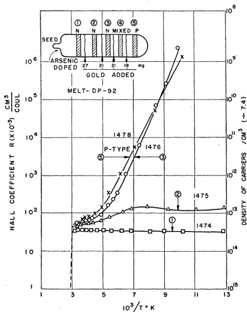
FIG. 1. Hall coefficient vs  $1/T^\circ\text{K}$  for a series of germanium samples cut from wafers containing progressively increasing amounts of gold. The crystal was originally *n*-type before gold was added. Each successive wafer is more *p*-type as the result of the addition of gold, as well as the normal segregation process. The scale at the right represents  $(1/7.4)$  times the actual density of carriers.
