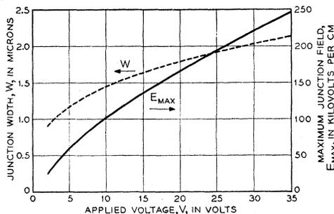
FIG. 5. Variation of junction width  $W$  and maximum junction field  $E_{\max}$  with applied voltage  $V$  for the germanium junction.
