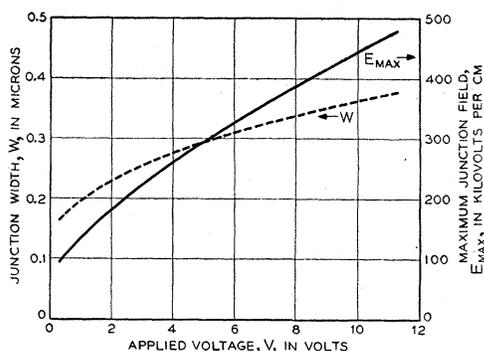
FIG. 4. Variation of junction width  $W$  and maximum junction field  $E_{\max}$  with applied voltage  $V$  for the silicon junction
