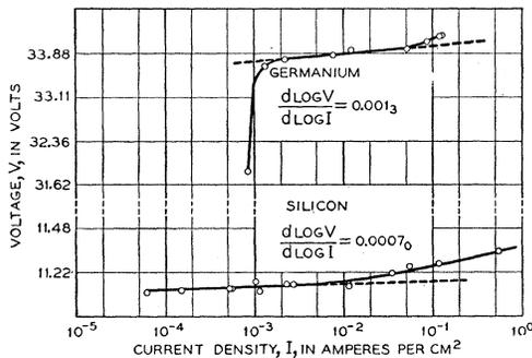
FIG. 2. Enlarged  $I/V$  characteristics, showing the details in the breakdown region.
