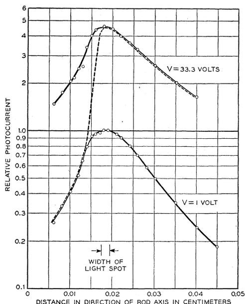
Fig. 7. Photoresponse of the germanium junction as a function of distance from junction of light spot for two different values of applied voltage. The dotted curve represents the expected response if holes injected by light did not multiply in junction.
