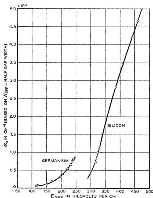
FIG. 10. Calculated ionization coefficients for germanium and silicon.
