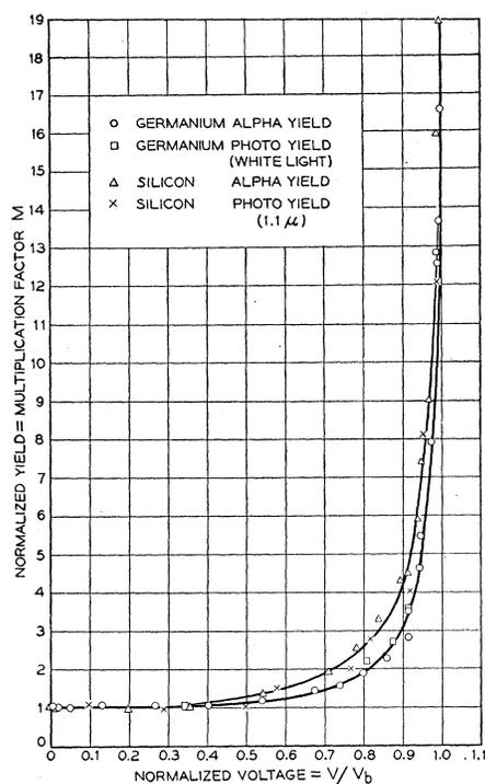
FIG. 9. Normalized yield curves of alpha bombardment and of photoconductivity for the silicon and germanium junctions from Fig. 8 and Fig. 6. Ordinate normalization was obtained by setting photo or alpha yield equal to unity for small applied voltage. Abscissa normalization was obtained by dividing the applied voltages by the breakdown voltages from Fig. 2.
