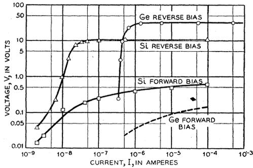
FIG. 1. Current vs voltage characteristics for the germanium and silicon *p-n* junctions.
