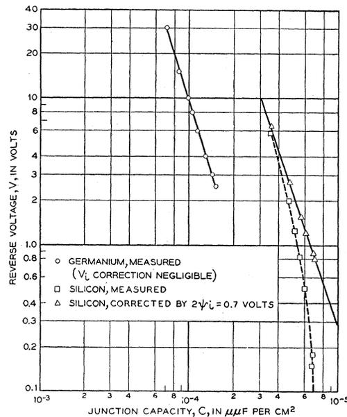
FIG. 3. Measured variation of junction capacity with applied voltage.
