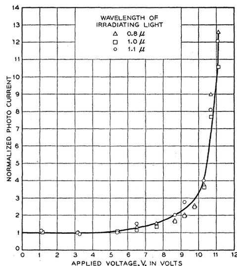
FIG. 6. Variation of photocurrent with applied junction voltage for light of various frequencies illuminating the silicon junction. The ordinate scales have been normalized by setting the photocurrent equal to unity at low voltages.
