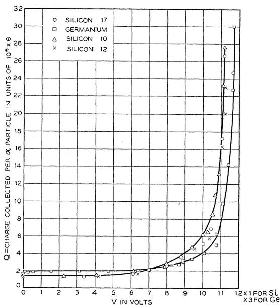
Fig. 8. Charge  $Q$  collected per alpha particle incident on junction of applied voltage. Data are shown for three separate silicon junctions and the germanium junction. Silicon No. 10 is the junction used in all other figures.
