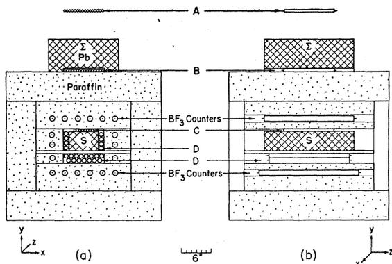
FIG. 1. Geometry of experiment.
