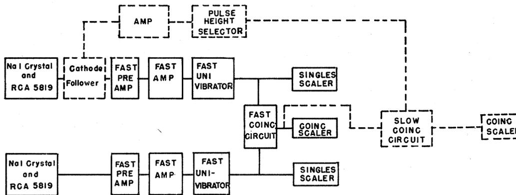
FIG. 1. Block diagram of electronic circuit.
