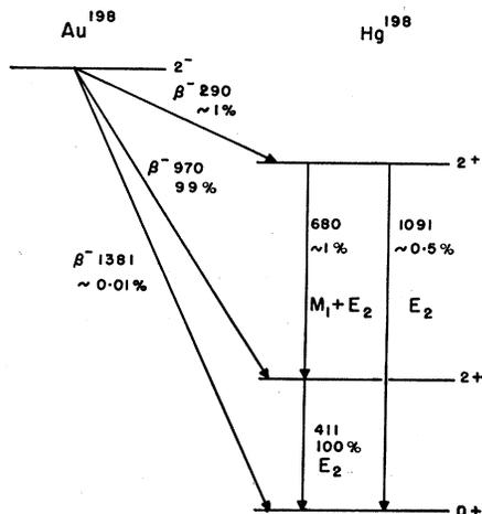
FIG. 4. Au<sup>198</sup> decay scheme.
