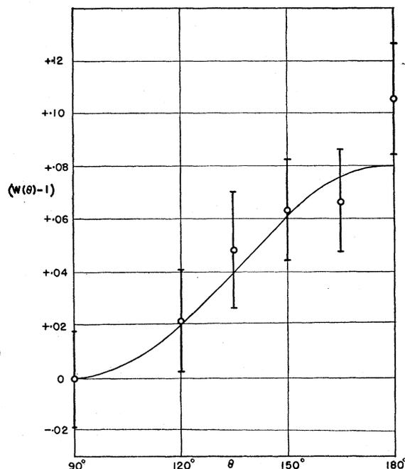
FIG. 3.  $\text{Fe}^{59}$  directional correlation. Data corrected for angular resolution.
