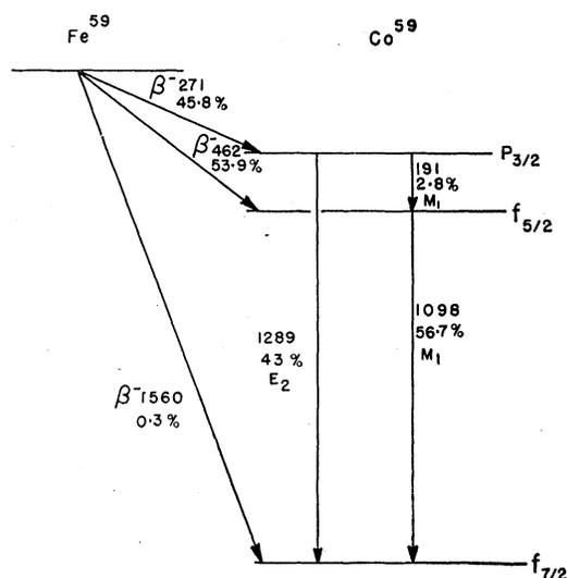
FIG. 2.  $\text{Fe}^{59}$  decay scheme.
