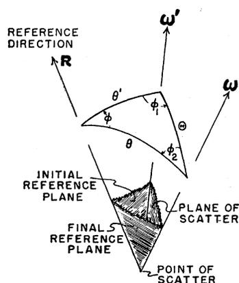
FIG. 1. The geometry of a Compton scattering. A photon traveling initially in the direction  $\omega'$  is scattered into a new direction  $\omega$ . The plane of scatter includes the two photon directions, and the initial and final reference planes relate  $\omega'$ ,  $\omega$  to a reference direction  $R$ .
