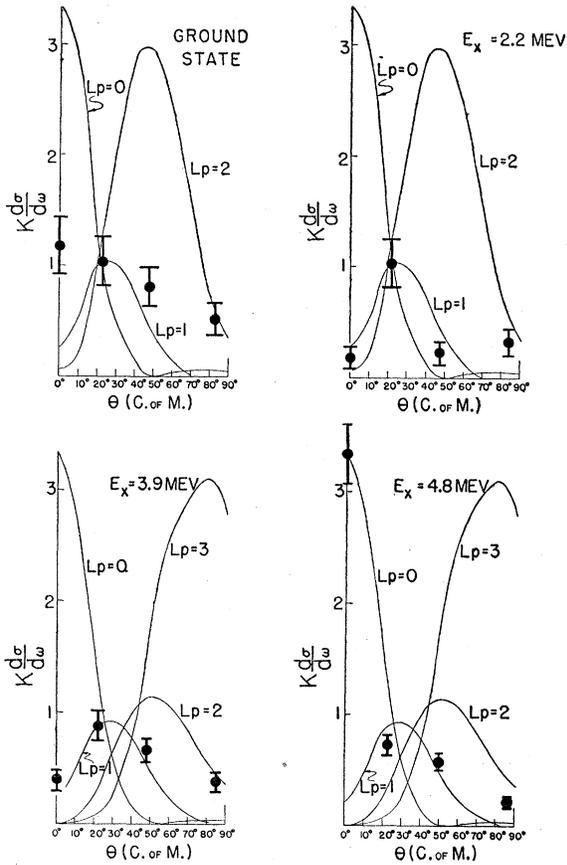
FIG. 3. Angular distributions of neutrons from the lowest four states of  $N^{14}$ . Center-of-mass coordinates. Solid curves are calculated from Butler theory.
