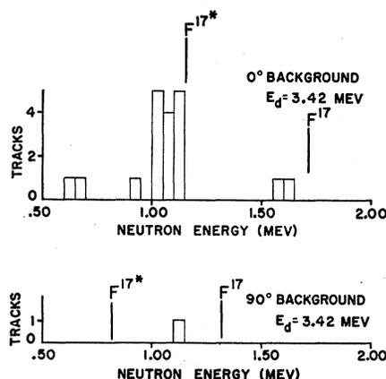
FIG. 7. Histograms of  $0^\circ$  and  $90^\circ$  background plates for the  $(d,n)$  exposure. The  $90^\circ$  histogram represents a plate area one-half that for the  $0^\circ$  histogram. Also indicated are the calculated positions for neutrons from the  $O^{16}(d,n)F^{17}$ ,  $F^{17*}$  reactions.
