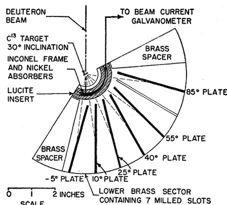
Fig. 1. Plate camera at midsection showing arrangement of the photographic emulsions for the  $C^{13}(d,p)C^{14}$  exposure.
