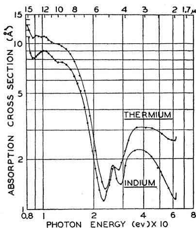
FIG. 2. Absorption cross section vs wavelength curves for chemically indium *P*-doped germanium and for strongly thermiated germanium.
