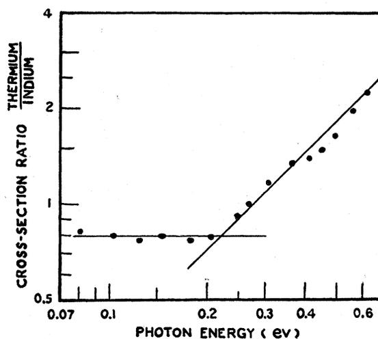
FIG. 3. Absorption cross-section ratio calculated from data of Fig. 2 plotted against photon energy in ev.
