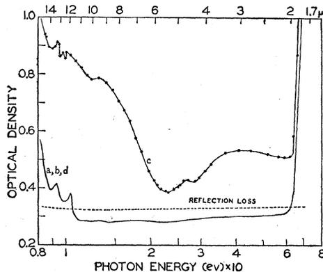
FIG. 1. Curve marked  $a$ ,  $b$ ,  $d$  represents the identical optical density vs wavelength curves obtained for germanium samples  $a$ ,  $b$ , and  $d$ , respectively. Curve  $c$  represents the results obtained with the thermiated germanium sample  $c$ . The dotted curve was calculated from refractive index data.
