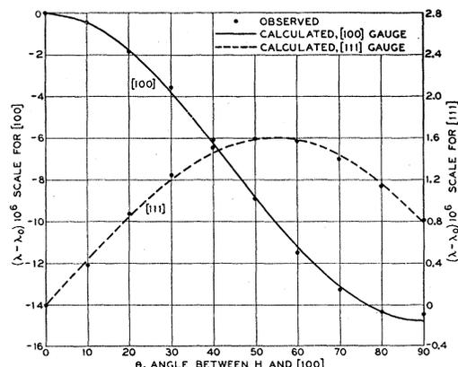
FIG. 1. Comparison of observed values of  $\lambda_i = \lambda - \lambda_0$  with those calculated from  $h_1, \cdots, h_5$  for least square fit.  $\lambda$ 's were measured parallel to [100] and [111] directions.
