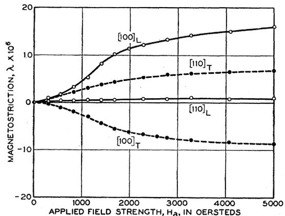
FIG. 2. Magnetostriction vs field strength for  $\text{Fe}_2\text{NiAl}$  (Mishima alloy), showing  $\lambda_l$  (longitudinal) with same sign as  $\lambda_t$  (transverse).
