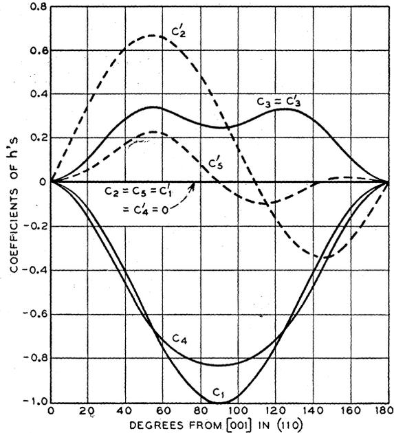
FIG. 3. Coefficients  $c_1, c_2, \dots, c_5$  of the terms in  $h_1, \dots, h_5$  of Eq. (1), for  $\lambda$  measured in (110) plane parallel to  $[001]$  (unprimed  $c$ 's) and to  $[111]$  (primed  $c$ 's), with magnetization at  $\theta^\circ$  from  $[001]$ .
