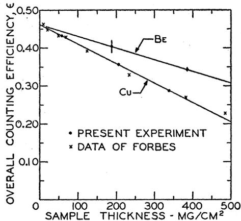
FIG. 2. Variation with sample thickness of the effects of self-scattering and absorption of beta-rays in copper and beryllium.
