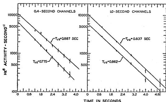
Fig. 4. Decay of  $\text{He}^6$  activity induced in Be by 14-Mev neutrons.
