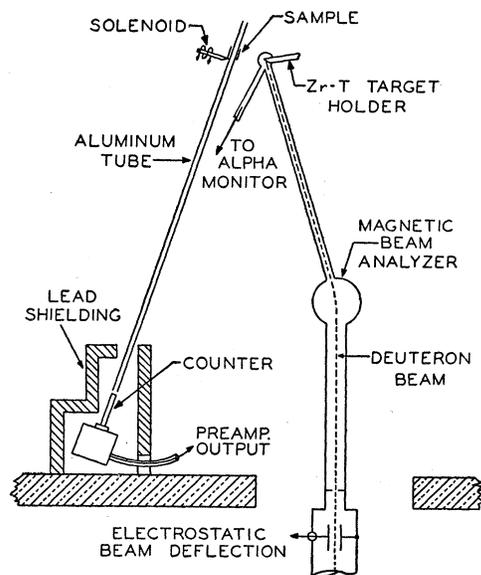
FIG. 1. Experimental arrangement for  $(n, \text{He}^6)$  cross-section measurements.
