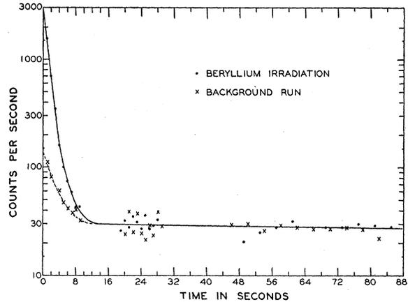
FIG. 3. Upper curve: Decay of He<sup>6</sup> activity induced in Be by 14-Mev neutrons, background included. Lower curve: Decay of background activity.
