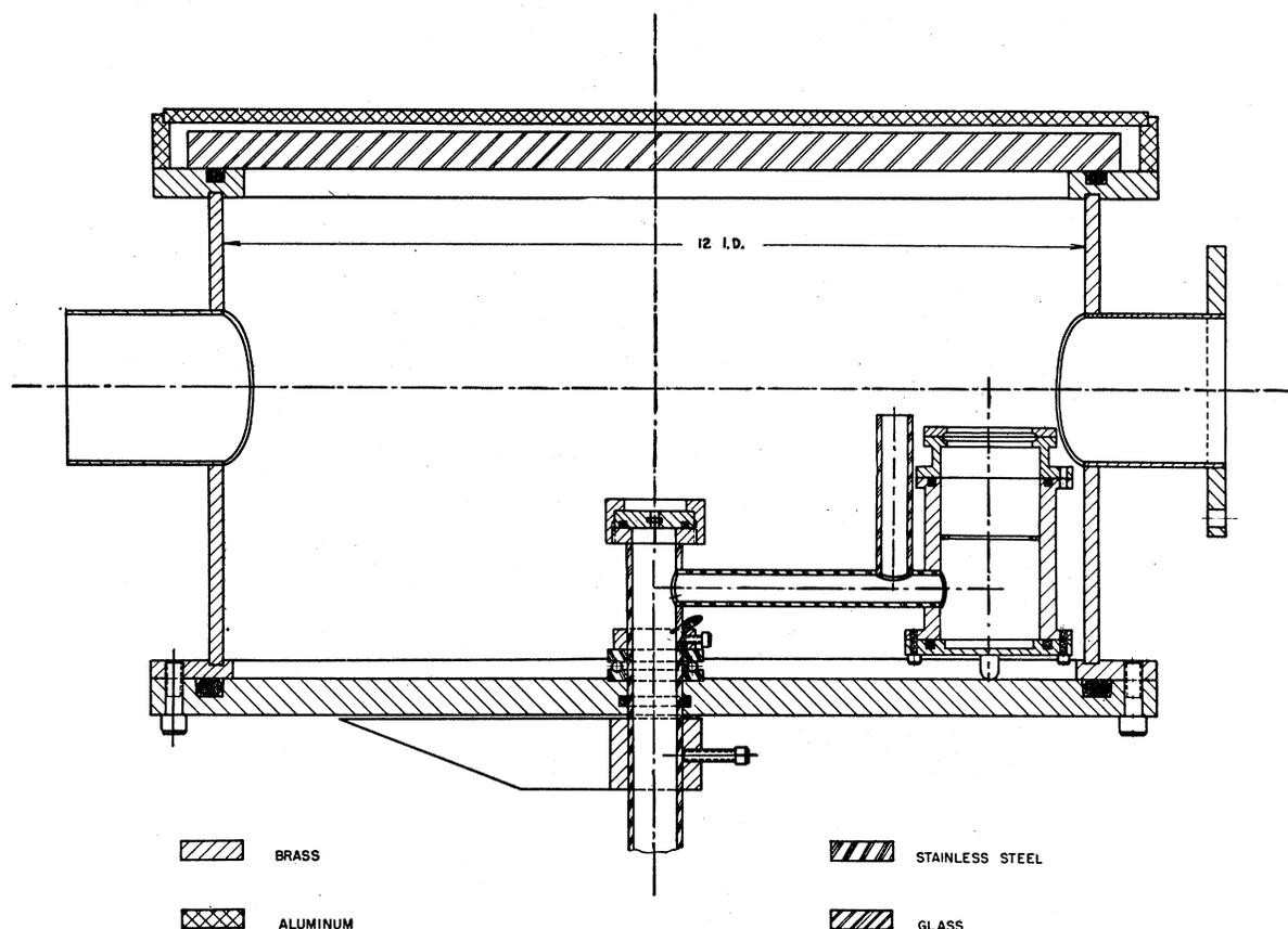
FIG. 2. Side view of the scattering chamber.
