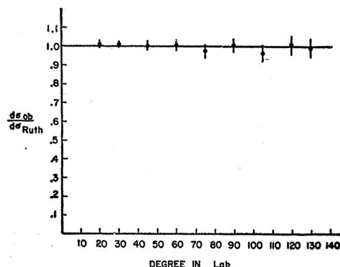
FIG. 6. Angular distribution of elastic scattering of 6.5-Mev protons from gold.
