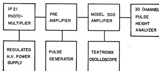
FIG. 3. Block diagram of the electronic apparatus.
