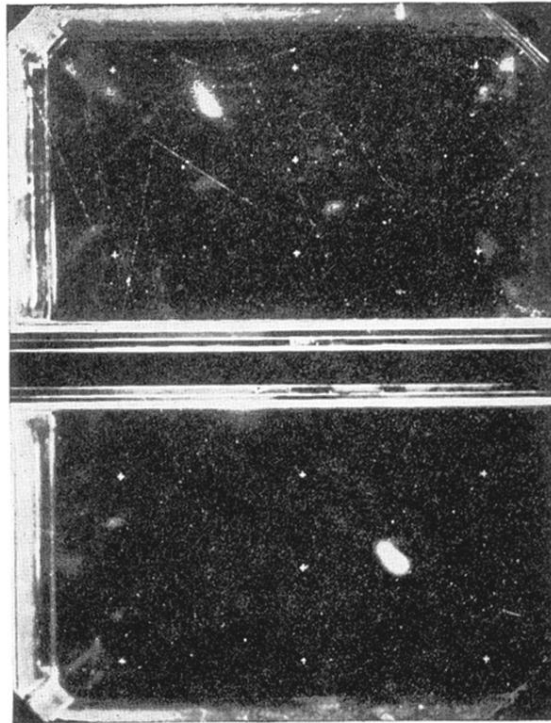
FIG. 16. Example of V^0 decay leading to a positive meson (presumably a \pi -meson) and a negative particle whose mass is considerably greater than that of a \pi -meson. The decay is in the upper left part of the upper chamber; the positive particle proceeds downward from the decay point, and the negative, toward the right and slightly downward.
