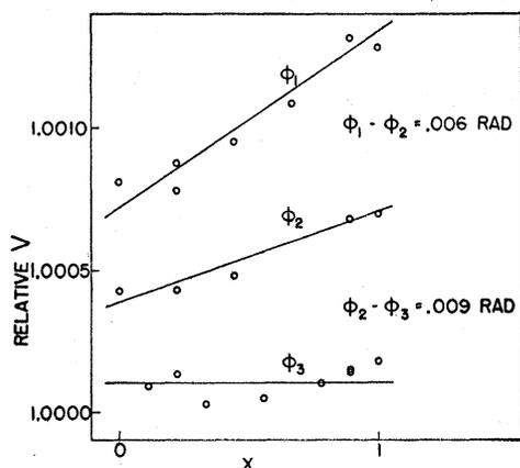
FIG. 2. Velocity-selector voltage  $V$  to focus electrons as a function of scanning-slit position  $x$  for three different values of momentum-selector angle  $\phi$ . (The aperture  $H$  has unit width in  $x$  on this plot.)
