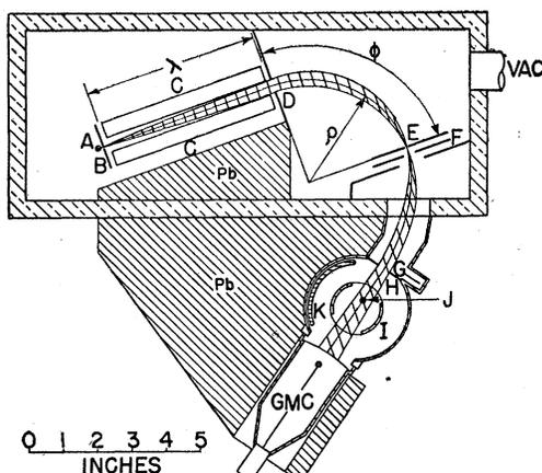
FIG. 1. Plan view of double-focusing mass spectrometer. Spacing between plates  $CC$  and the widths of slits  $B$ ,  $E$ , and rough-slit  $D$  are grossly exaggerated in order to show a bundle of particle trajectories. The magnetic field is uniform over the rectangular part of the vacuum chamber and is out of the paper. The vacuum chamber height between magnet pole faces is  $1\frac{1}{8}$  in.
