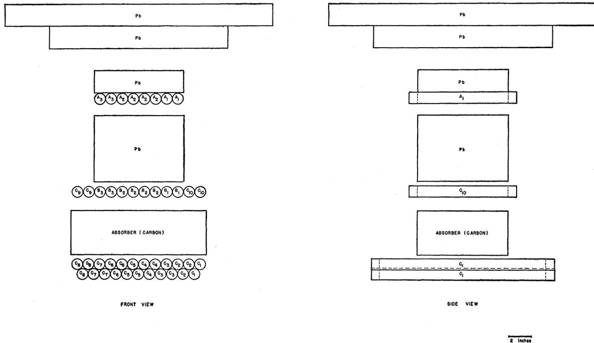
FIG. 1. Diagram of apparatus. The mesons actually recorded were those which, after crossing the counter telescope, were stopped in the graphite absorber and decayed between about 1.2 and 7  $\mu$ sec into electrons discharging counters C.
