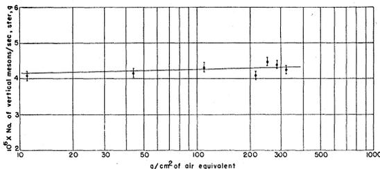
FIG. 2. The differential range spectrum of sea-level mesons at Rio Piedras, Puerto Rico—geomagnetic latitude  $29^\circ\text{N}$ . The absolute number of mesons per sec sterad  $g$  is represented as a function of their range expressed in  $g/\text{cm}^2$  of air equivalent.
