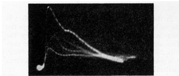
FIG. 19. \alpha -particle pulses in argon plus mercury vapor at the corona threshold. Pressure=1000 mm Hg; markers=1 \mu sec; RC=1 \mu sec. The slow decay is due to production of electrons in the gas.
