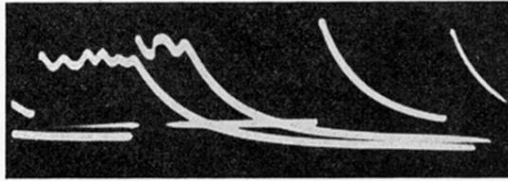
FIG. 15. Bursts in unstable corona zone. Argon plus \sim 10^{-2} carbon dioxide; counter diameter = 130 mm; pressure = 760 mm Hg; sweep time = 30 msec; RC = 200 \mu\text{sec} .
