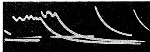
FIG. 15. Bursts in unstable corona zone. Argon plus \sim 10^{-3} carbon dioxide; counter diameter = 130 mm; pressure = 760 mm Hg; sweep time = 30 msec; RC = 200 \mu\text{sec} .
