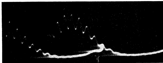
FIG. 11. \beta -pulses in the Geiger zone. Argon plus \sim 10^{-3} carbon dioxide; pressure=760 mm Hg; sweep time=50 \mu sec; RC=1 \mu sec.
