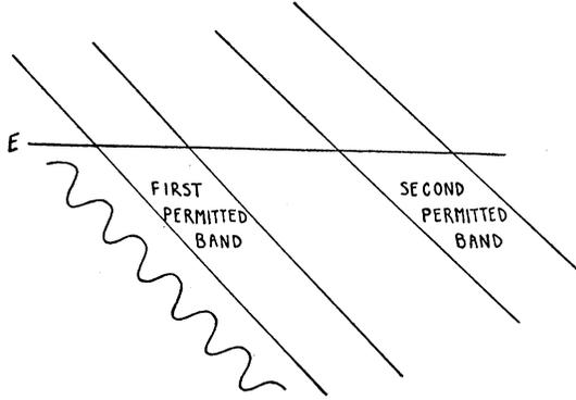
FIG. 1. Potential and energy bands in a periodic potential perturbed by a linear potential.
