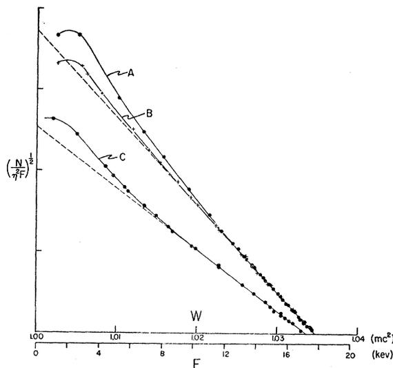
FIG. 4. Fermi plots obtained with sources reversed so that the Zapon support was between the activity and the detector.
