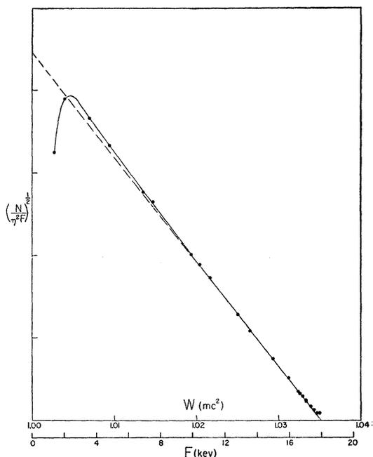
FIG. 3. Fermi plot of the tritium spectrum data obtained with a source which was grounded by a  $2\mu$  g/cm<sup>2</sup> Cu deposit on the backing.
