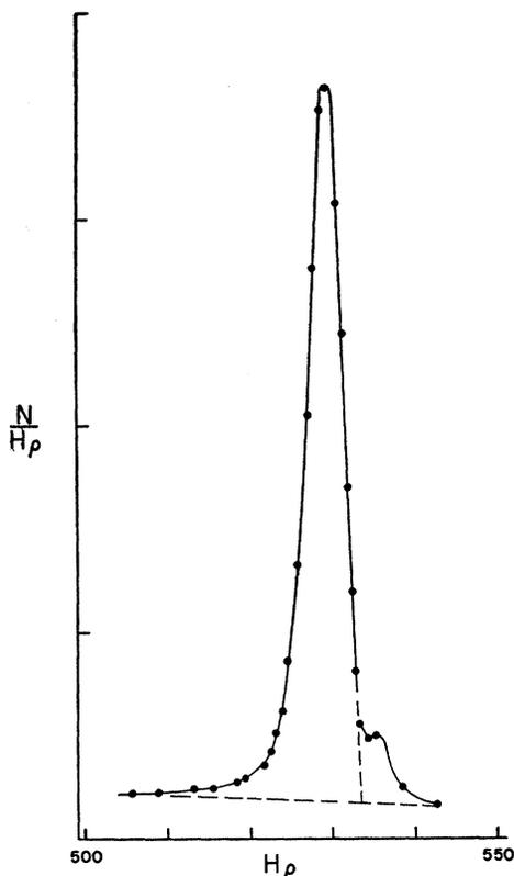
FIG. 1. Typical momentum profile obtained for the "A" line of ThC<sup>232</sup> used for calibration.
