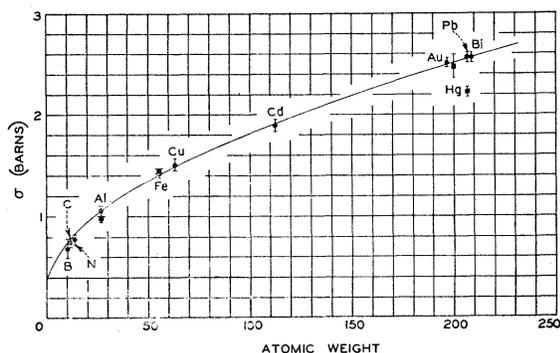
FIG. 1. Inelastic collision cross sections for 14-Mev neutrons measured with copper threshold detectors plotted against atomic weights. The smooth curve was calculated from the empirical relation  $\sigma = \pi R^2$ , where  $R = (2.5 + 1.1 A^{1/2}) \times 10^{-13}$  cm. The squares are values of Amaldi *et al.* taken from reference 4.
