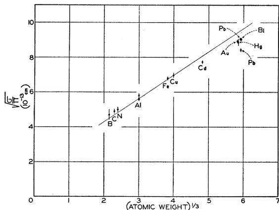
FIG. 2. Experimental values of  $(\sigma/\pi)^{1/2}$  as a function of the one-third power of the atomic weights. Solid circles represent data presented here. Crosses represent the data of Amaldi *et al.* taken from reference 4. The curve is calculated from the theory of Feshbach and Weisskopf.
