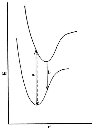
FIG. 2. Typical potential curve relationship.  $a$  = energy required to excite molecule;  $b$  = energy available after loss of upper state vibrational energy; dotted line = energy available for transfer before vibrational energy is lost.
