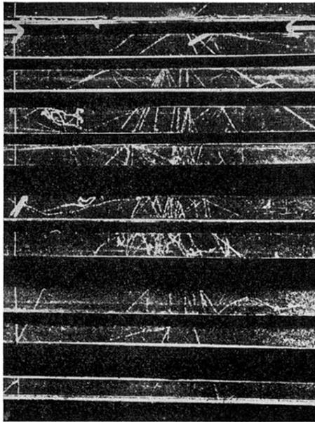
FIG. 7. A representative cloud-chamber photograph. The crystal plate is indicated by the arrows. This is a nuclear event in which no p.p. and one  $\pi^0$  were created. The two electromagnetic cores are clearly due to photons: the  $\pi^0$  had an energy higher than 1000 Mev.
