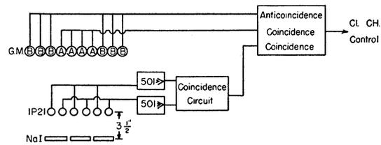
FIG. 2. Block diagram of the circuits and counters used for triggering the cloud chamber.
