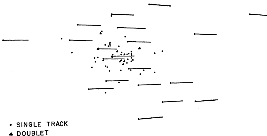
FIG. 8. Target diagram of the charged shower particles produced by an interaction in brass of an energetic cosmic-ray \alpha -particle (shower A of Table I). The shower particles are projected onto a plane perpendicular to the shower axis.
