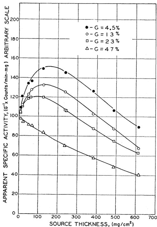
FIG. 1. Effect of sample thickness on apparent specific activities for Cu<sup>64</sup> beta-rays in copper foils for the three Geiger-counter geometries of 4.5, 13, and 23 percent, and for the 47 percent proportional counter geometry.
