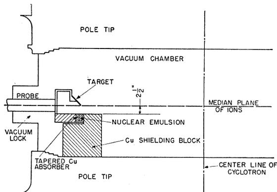
Fig. 1. Cross section view of cyclotron vacuum chamber.
