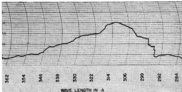
FIG. 2. Band emission curve of chromium.  $E_b=600$  volts,  $I_b=3$  ma.
