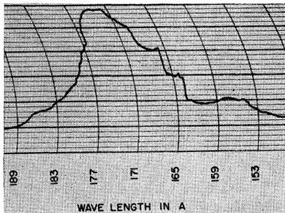
FIG. 1. Band emission curve of copper.  $E_b=500$  volts,  $I_b=3$  ma.
