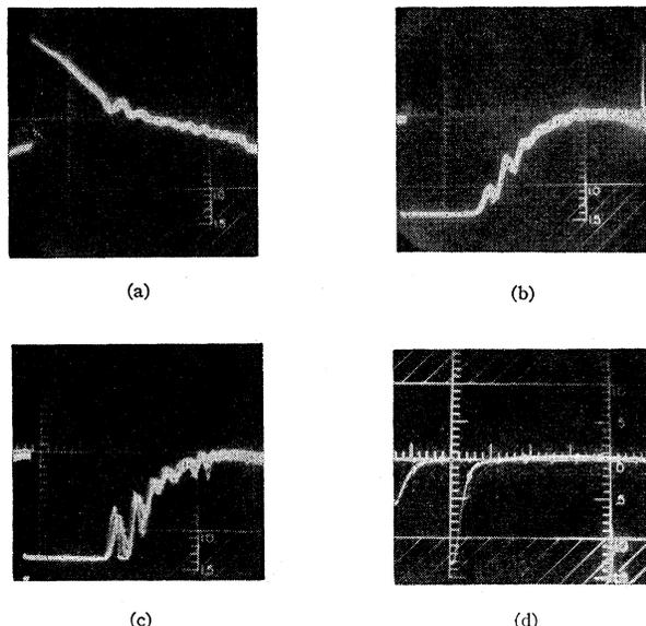
FIG. 1. Oscillations on current to probe in He at a pressure of 0.020 mm. The examining interval begins 600 microseconds after the excitation pulse. (a) Positive-ion current,  $H_0 = 530$  gauss; (b) electron current,  $H_0 = 530$  gauss; (c) electron current,  $H_0 = 410$  gauss; (d)  $H_0 = 0$ , when no oscillations occur anywhere in the afterglow period.
