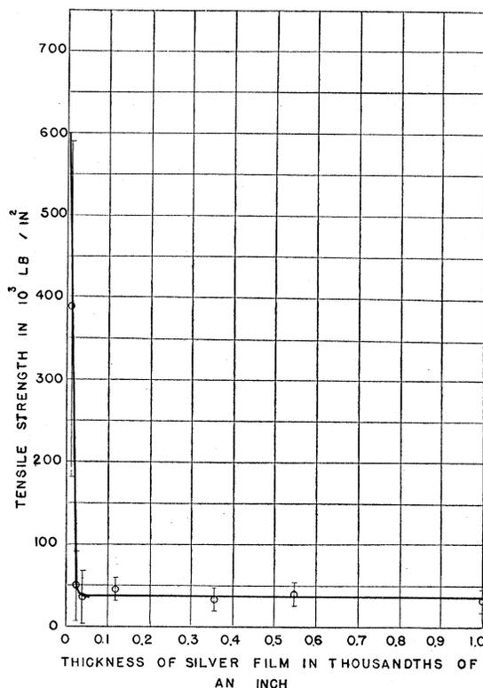
FIG. 1. Tensile strength as function of thickness.
