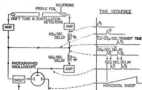
FIG. 1. Schematic diagram of the time-of-flight equipment. The time sequence illustrates that the less frequent pulses  $P_1$  from the fragments which travel the length of the drift tube initiate the oscilloscope display, the pulses  $P_0$  from the complementary fragments are delayed by the maximum transit time, and the mixture of  $P_1$  and  $P_0$  are, in addition, delayed for proper oscilloscope presentation.
