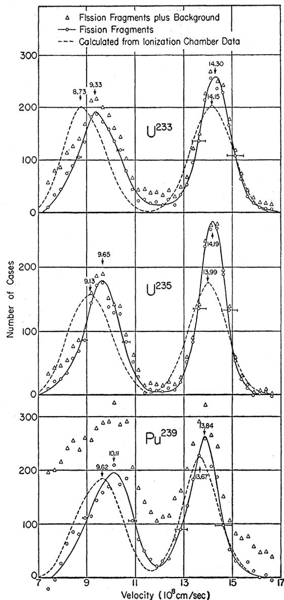
Fig. 2. Comparison of the velocity distribution of fission fragments with the distribution inferred from ionization chamber data. All distributions are normalized. Horizontal lines through the data represent half-widths of the resolutions of the velocity measurements. The large background in the  $\text{Pu}^{239}$  data is due to the large alpha-activity of  $\text{Pu}^{239}$ .
