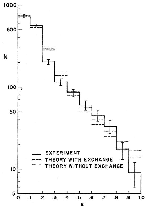
FIG. 3. The number,  $N$ , of positron-electron scattering events as a function of the fraction,  $\epsilon$ , of the positron's energy that is transferred to the electron. These results are for the present experiment.
