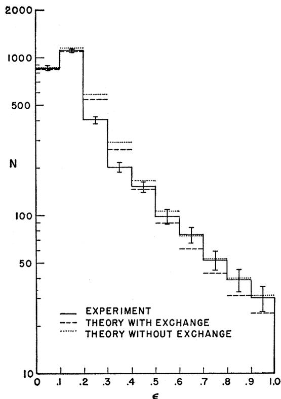
FIG. 4. The summation of the results of all experiments to date.  $N$  is the number of positron-electron scattering events, and  $\epsilon$  is the fraction of the positron's energy that is transferred to the electron.
