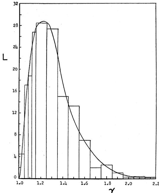
FIG. 2. Energy spectrum of the positrons used.  $L$  is track length in meters;  $\gamma$  is the positron energy in units of the electron rest energy. Multiply by 20.22 to find the total track length.
