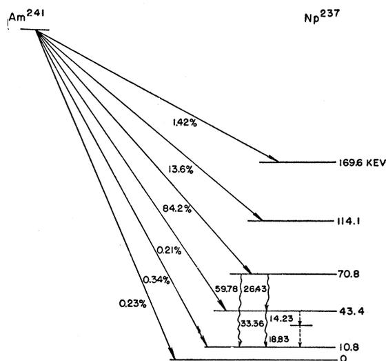
FIG. 6. Partial decay scheme for Am<sup>241</sup>. Energy levels shown were obtained from alpha-spectra. Gamma-ray energies shown were obtained with a bent crystal spectrometer (see reference 14).
