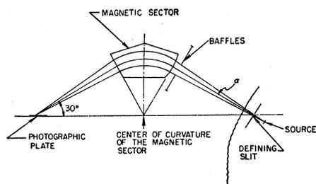
FIG. 1. Schematic diagram of the optics of the spectrograph.
