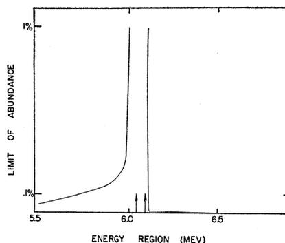
Fig. 8. Upper limit of abundance of alpha-groups of Cm<sup>242</sup> as a function of energy (arrows indicate positions of known alpha-groups).
