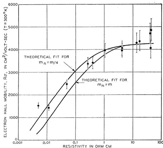
FIG. 1. Electron hole mobility in Ge as a function of resistivity.
