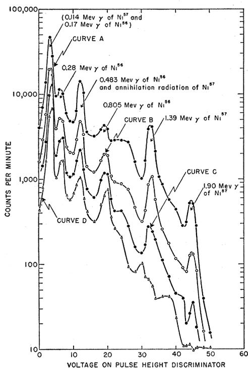
FIG. 1. Gamma-ray spectra of  $\text{Ni}^{56}$  and  $\text{Ni}^{57}$  as a function of time.
