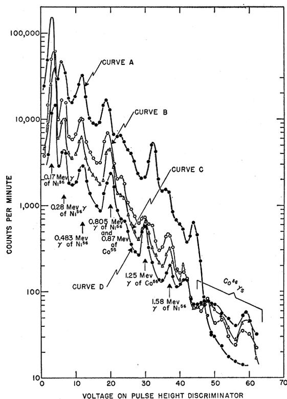
FIG. 2. Gamma-ray spectra of  $\text{Ni}^{56}$  (with a small amount of  $\text{Ni}^{57}$  present) and  $\text{Co}^{56}$  growing in.
