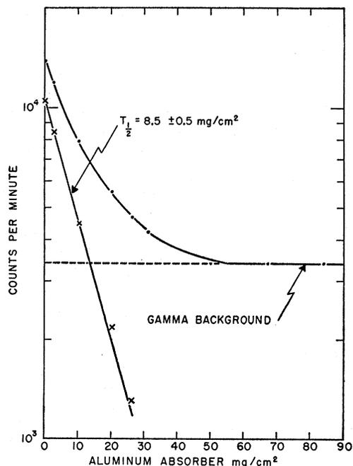
FIG. 3. Absorption of Ni<sup>56</sup> radiations by aluminum.
