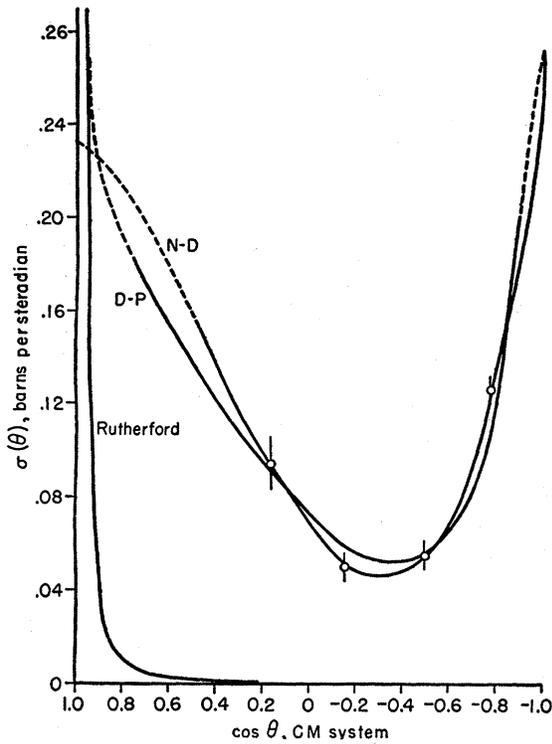
FIG. 1. Differential cross sections: 4.7-Mev  $n$ - $d$ , 10.4-Mev  $d$ - $p$ , and 5.2-Mev Rutherford.
