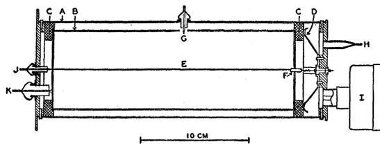
FIG. 2. Constructional details of ionization chamber. A, pressure vessel (0.032-in. Cu); B, cathode (0.032-in. Cu); C, cathode insulating rings (Mykroy); D, retaining spring; E, electron collector (0.010-in. Kovar); F, glass insulator; G, Po- $\alpha$  source electrode; H, pinch seal; I, 0–100 lb/in.<sup>2</sup> pressure gauge; J, connection to amplifier; K, —300 v cathode connection.
