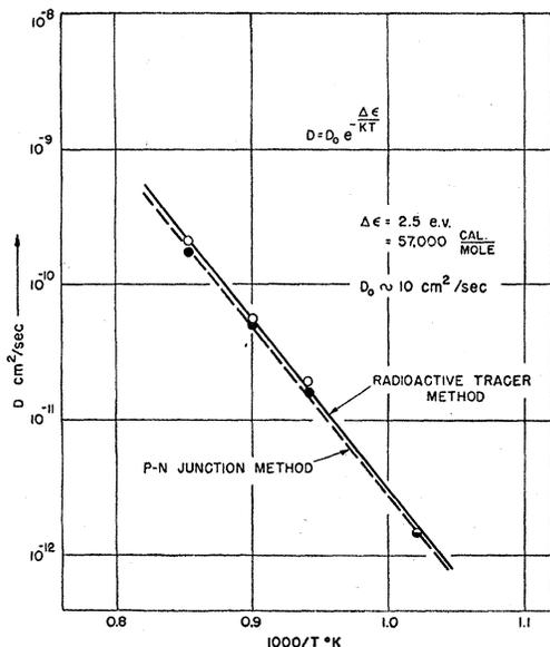
FIG. 2. Plot of the temperature variation of the diffusion coefficient for antimony in germanium determined by the  $p-n$  junction method and by the radioactive tracer method. The good agreement observed justifies the use of the  $p-n$  junction method for the measurement of diffusion in semiconductors.
