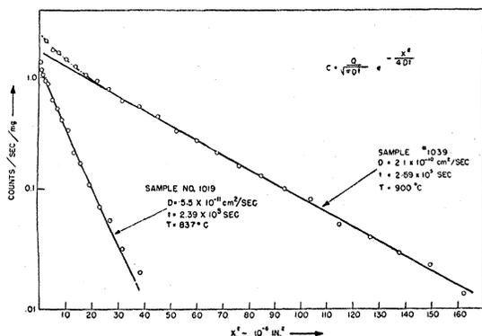
FIG. 1. Plot of  $\log$  (counting rate) vs  $x^2$  for the diffusion of radioactive antimony 124 into a germanium single crystal at two temperatures, 900°C and 837°C. The linearity of the plot on this chart is a test of the applicability of the " $\delta$ -function" solution of the diffusion equation.
