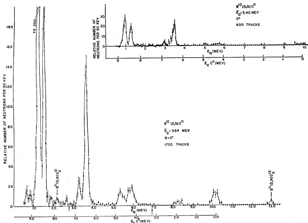
FIG. 1. Neutron spectrum at  $0^\circ$  from deuterons on 96 percent enriched  $B^{10}$  target. Upper curve: 3.40-Mev deuterons; lower curve: 3.64-Mev deuterons.
