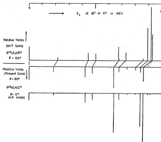
FIG. 6. Relative intensities of neutron and proton groups from  $B^{10}(d,p)B^{11}$  and  $B^{10}(d,n)C^{11}$ .
