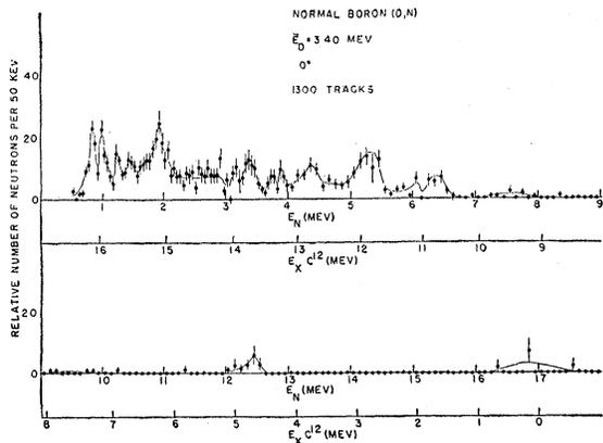
Fig. 2. Neutron spectrum at  $0^\circ$  from 3.40-Mev deuterons on normal boron target.
