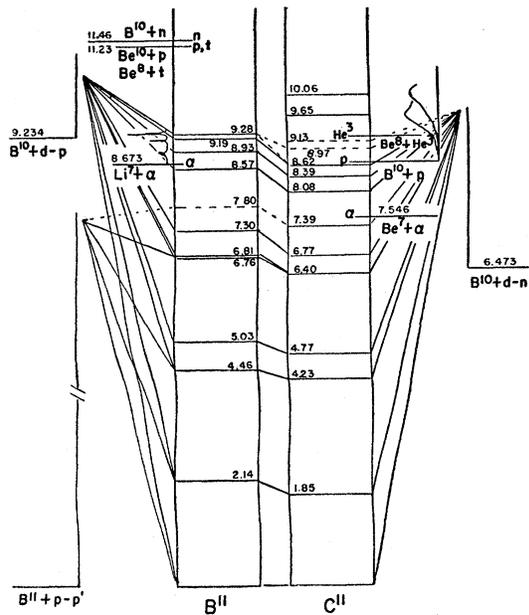
FIG. 5. Comparison of levels of  $B^{11}$  and  $C^{11}$  (ground state of  $C^{11}$  normalized to  $B^{11}$  ground state).
