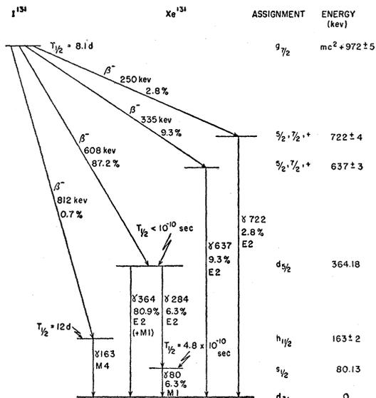
FIG. 7. Proposed disintegration scheme of  $I^{131}$ . The detailed properties of the beta-components and gamma-rays are explained in the text and listed in Tables I and II. The orbital assignments are made from experimental results and are consistent with the nuclear shell model. Most of the published observations on  $I^{131}$  can be reconciled with this scheme.
