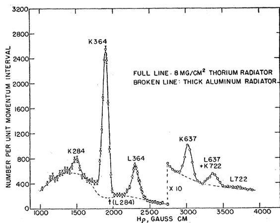
Fig. 4. Secondary electron spectrum of  $Xe^{131}$  gamma-rays from an  $I^{131}$  source using a Th radiator, 8 mg/cm<sup>2</sup>. The shape of the spectrum observed with the Th radiator removed, leaving a thick Al radiator, is indicated by a broken line. Where the standard deviations of the points are greater than the radii of the circles, they are indicated by vertical bars.
