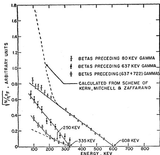
FIG. 6. Coincidence Fermi plots for  $I^{131}$ . Upper curve, spectrum of coincidences between beta-rays and 80-keV gamma-rays; the broken line shows what would be expected on the disintegration scheme of Kern *et al.*, reference 4. Middle curve, spectrum of coincidences between beta-rays and 637-keV gamma-rays. Lower curve, spectrum of coincidences between beta-rays, and an equal mixture of 637- and 722-keV gamma-rays. The standard deviations of the points are shown by vertical bars.
