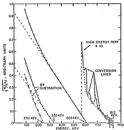
FIG. 3. Allowed Fermi plot of the beta-ray spectrum of  $\text{I}^{131}$  as observed in Fig. 2. For the part below 570 keV, the conversion lines were omitted as indicated by broken lines in Fig. 2. Where the standard deviations of the points are greater than the radii of the circles, they are indicated by vertical bars. Since the errors of the subcomponents ending at 335 and 250 keV are probably chiefly systematic, no attempt has been made to indicate standard deviations for them.
