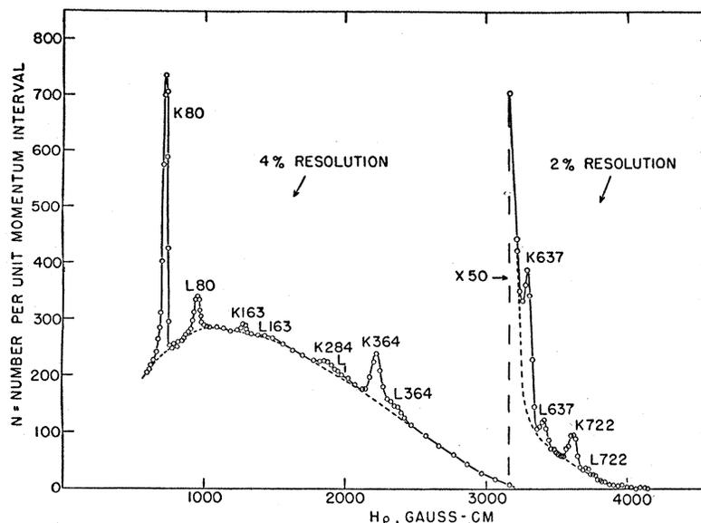
FIG. 2. Observed beta-ray spectrum of  $I^{131}$ . The right-hand part of the spectrum was measured with higher resolution in the spectrometer. The standard deviations of the points are everywhere smaller than the radii of the circles.
