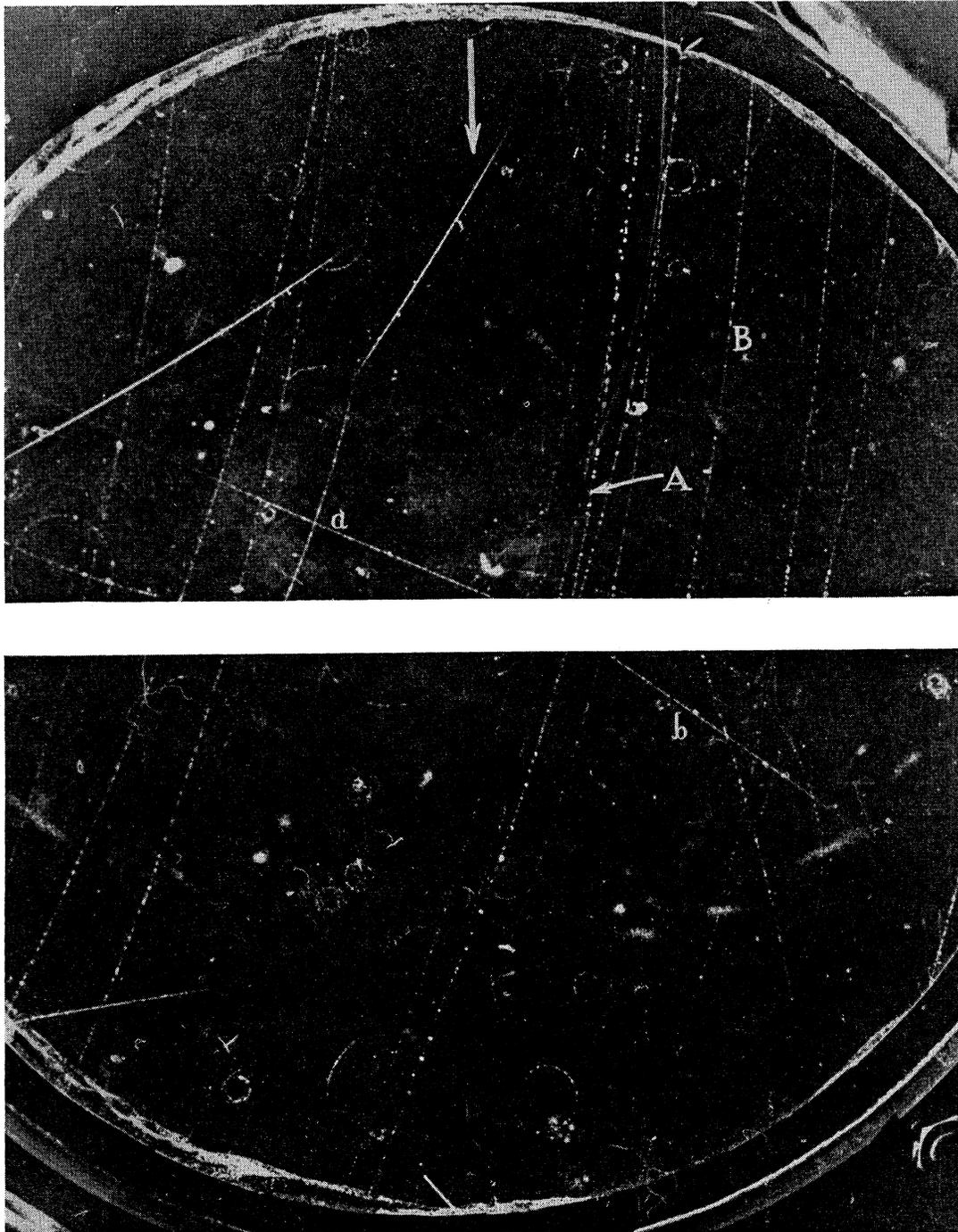
FIG. 1. 70-Mev  $\pi^+$  meson beam photograph. Meson *A* yields a 2-proton star, prongs *a* and *b*. Meson *B* elastically scatters through an angle of  $32^\circ$ .
