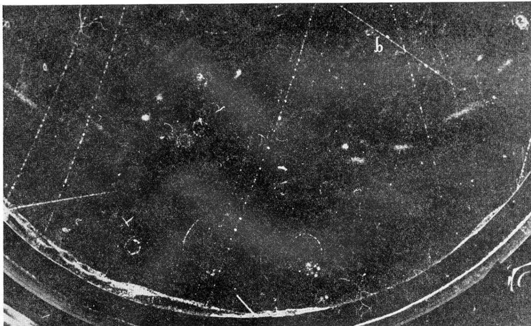
FIG. 1. 70-Mev  $\pi^+$  meson beam photograph. Meson *A* yields a 2-proton star, prongs *a* and *b*. Meson *B* elastically scatters through an angle of  $32^\circ$ .
