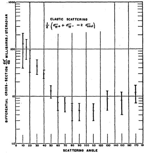
FIG. 4. Differential elastic scattering cross section for pions on carbon obtained by averaging the  $\pi^+$  and  $\pi^-$  results and subtracting the contribution of a uniformly charged sphere (Born approximation).
