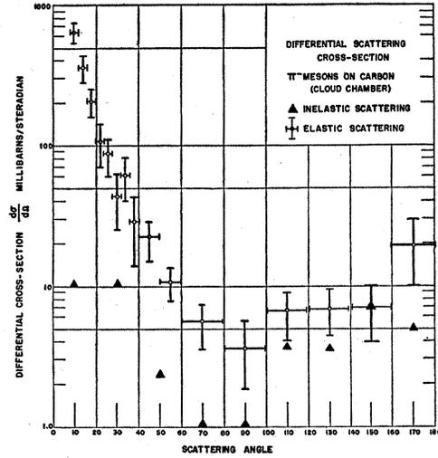
FIG. 2. Differential elastic and inelastic scattering of negative pions on carbon.
