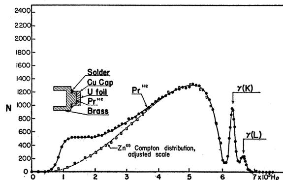
FIG. 1. The solid line, given by the circles, is the secondary electron spectrum of  $\text{Pr}^{142}$  as obtained with the arrangement shown in the insert. The broken line, given by squares, was obtained from the Compton distribution produced by the  $\text{Zn}^{65}$  gamma-ray (1.12 Mev) normalized to the Compton distribution from  $\text{Pr}^{142}$ .  $N$  is the number of counts per minute.
