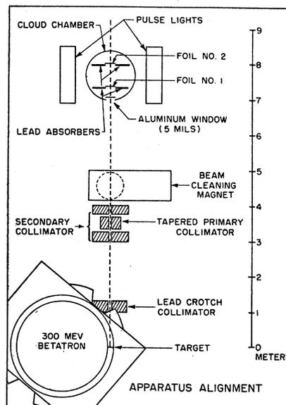
FIG. 2. The collimation scheme for obtaining a small beam in the chamber.
