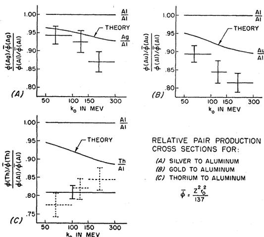
FIG. 5. Comparison of the calculated relative pair production cross sections with the experimentally observed values.
