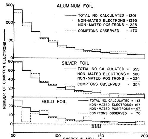
Fig. 3. Histogram showing both the calculated and observed number of Compton electrons from the Al, Ag, and Au foils.
