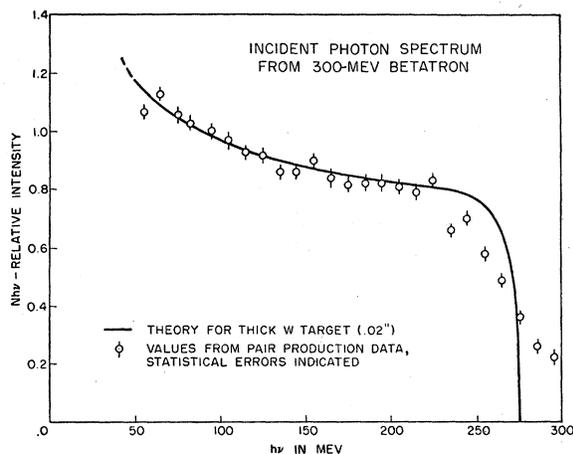
FIG. 6. Comparison of the thick target theoretical bremsstrahlung to the experimental points.
