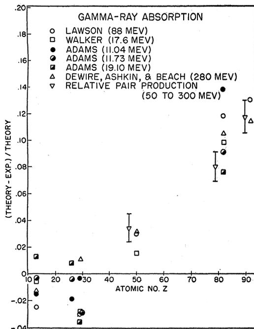
FIG. 7. A presentation of the gamma-ray absorption discrepancy between theory and experiment as found by several experimenters. Relative pair production discrepancies are also shown for comparison.
