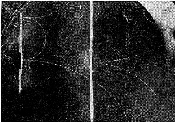
FIG. 1. Photograph of the cloud-chamber showing pairs created in Au and Al foils by a beam of photons traversing the chamber from left to right. Note Pb absorbers on which the foils were mounted.
