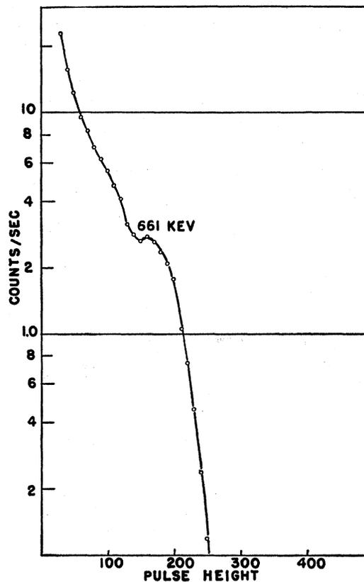
FIG. 2.  $Cs^{137}$   $\gamma$ -rays on LiI-SnI<sub>2</sub>. The pulse-height scale is twice that of Fig. 1.
