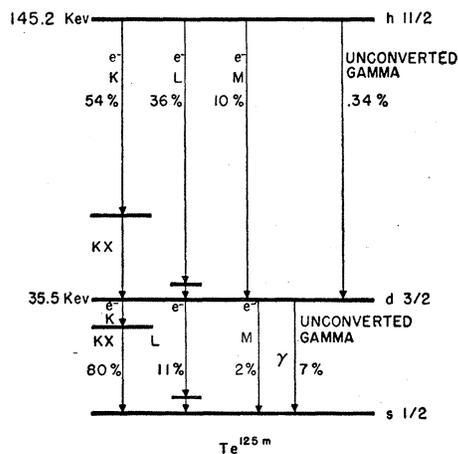
FIG. 1. Decay scheme of  $\text{Te}^{125m}$ .
