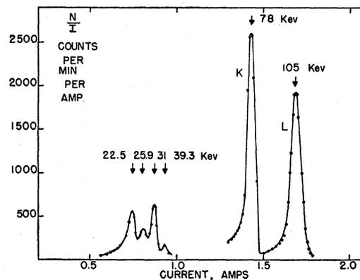
FIG. 3. Electron spectrum taken with lens spectrometer. The 78- and 105-keV lines are due to  $K$  and  $(L+M)$  conversion electrons from the 110-keV gamma-ray.
