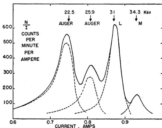
FIG. 6. Low energy electron spectrum taken with lens spectrometer. Dashed curves show the contributions of the four electron groups.
