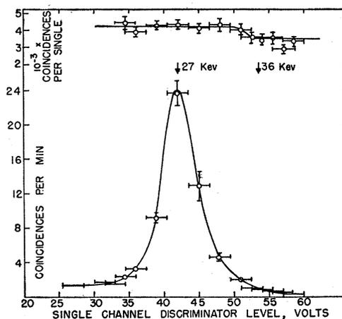
FIG. 5. Photon-photon coincidences. The channel level of one proportional counter is the abscissa. The selector of the other proportional counter detected one-half of the x-ray pulses.
