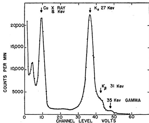
FIG. 4. Photon spectrum, proportional counter detector. The Cu x-ray originates in the counter wall.
