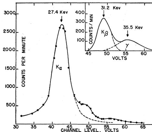
FIG. 7. Analysis of proportional counter photon spectrum.
