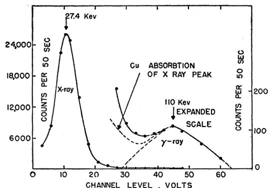
FIG. 2. Photon spectrum, NaI crystal detector. Expanded scale on right applies to gamma-ray. Partial absorption of x-ray by Cu shown by dashed curve. Note added in proof.—The expanded scale on the right of Fig. 2 is in error; the number of counts should be one-half of the values listed. This error was pointed out by Dr. A. W. Sunyar.
