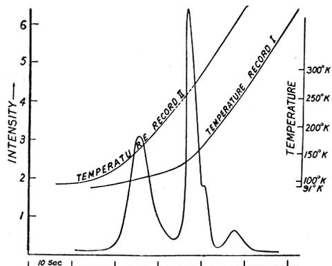
FIG. 1. Thermoluminescence curve of potassium iodide starting from liquid oxygen temperature, after excitation by cathode-rays at 10 kv for five minutes. The temperature record No. I corresponds to the thermoluminescence curve. The dotted part of temperature record No. II gives the temperature range at which coloration disappears on heating from 91°K after bombardment.
