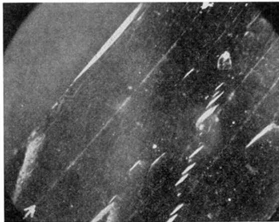
FIG. 2. Domain pattern on 11\bar{2} plane which was outer face of a leg of the sample. The movable wall is indicated by white arrows. The other walls did not extend as far along the leg, and are therefore identified with the break in the sample. The edge of the sample runs from the top of the picture toward the left.
